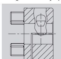
Frictionally engaged shaft-hub connection for radial assembly of couplings. Transmittable torque depends on the bore size (only for ATEX category 3)
