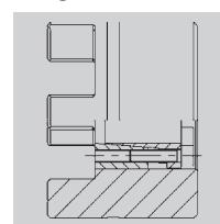
Frictionally engaged, zero-backlash shaft-hub connection for high torque. Largest clamping device possible depends on the hub O.D. Clamping device can be mounted on jaw side or back face. For details, see the CLAMPEX® section.
