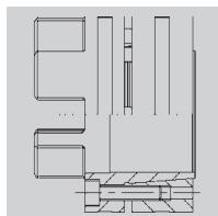
Integrated frictionally engaged shaft-hub connection for high torque. Fasteners are in the face of the hub. For details about torques and dimensions see page 32. Suitable for high speeds.
