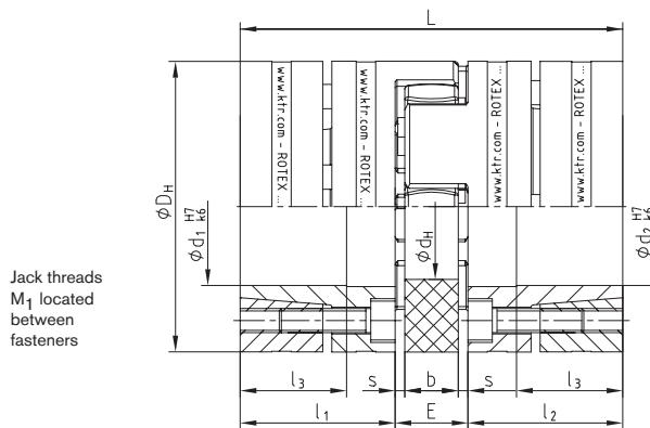
Inch bores machined to AGMA Class 1, Metric bores machined to H7 or G7 if greater than 55mm
