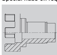
Special lengthened hub/shaft with integrated jaws.
