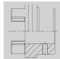
Positive torque transmission for pressed or glued connections. (No ATEX certification available)
