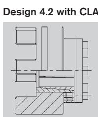
Frictionally engaged shaft-hub connection for average torque.
