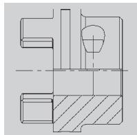
Frictionally engaged shaft-hub connection.
