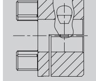
Frictionally engaged shaft-hub connection for radial assembly of couplings. Transmittable torque depends on the bore size (only for ATEX category 3).
