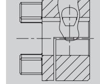
Positive power transmission with frictionally engaged operation for radial assembly of couplings. The frictionally engaged operation reduces backlash. Surface pressure of the keyway connection is reduced.
