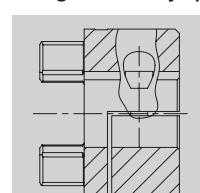
Positive torque transmission with keyway for radial assembly of couplings. Positive lock reduces backlash. Surface pressure of the keyway connection is reduced.
