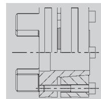
Design equal to 6.0, but fasteners are on the back face. Suitable for easy disassembly of intermediate shafts (special design).
