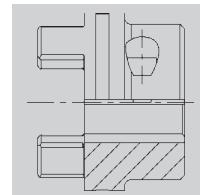
Positive torque transmission with additional frictional torque capacity. The additional frictional torque capacity reduces backlash. Surface pressure of the keyway is also reduced.
