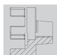
Special hub with an external taper for a frictional connection.
