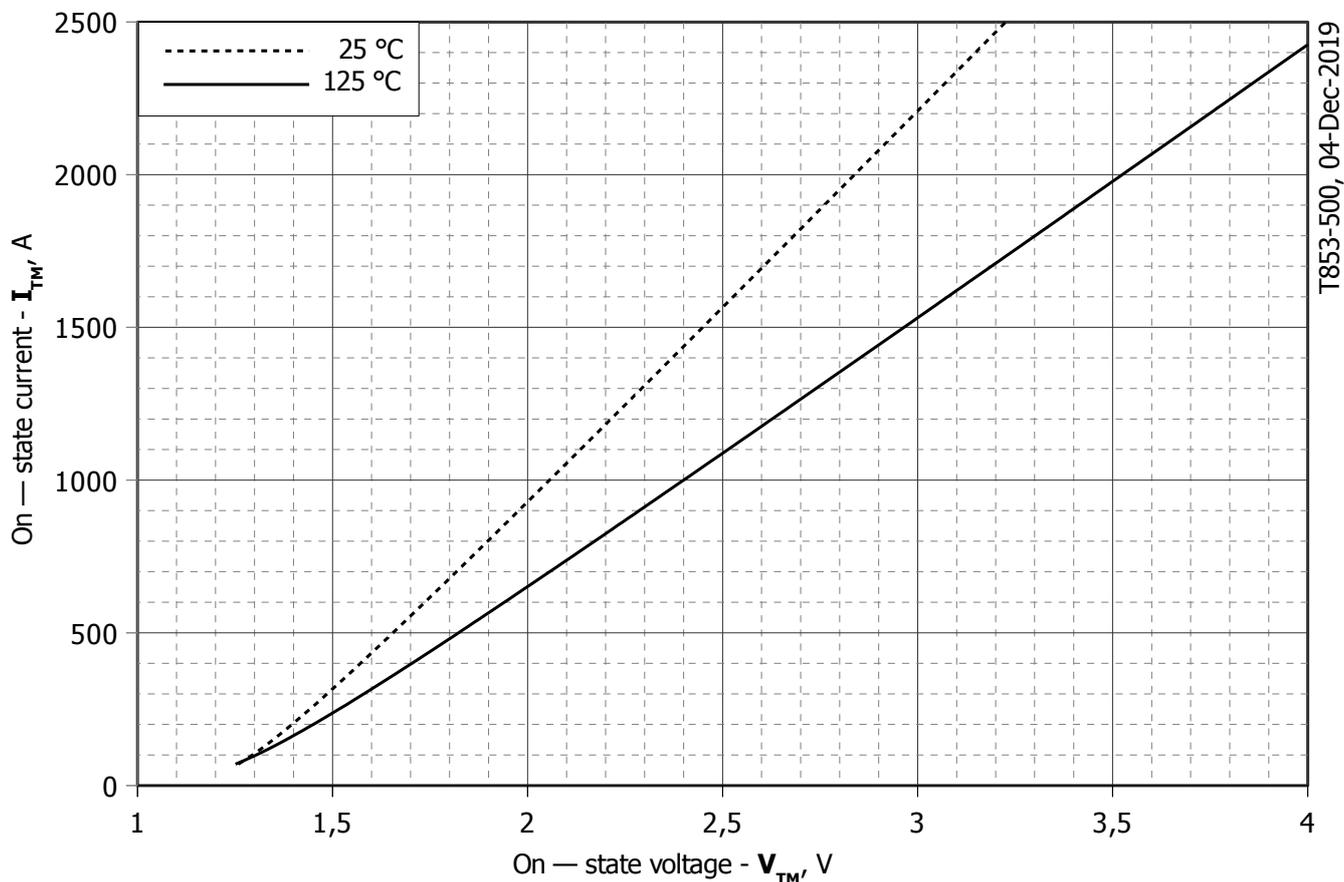
**Fig 1 – On-state characteristics of Limit device**
